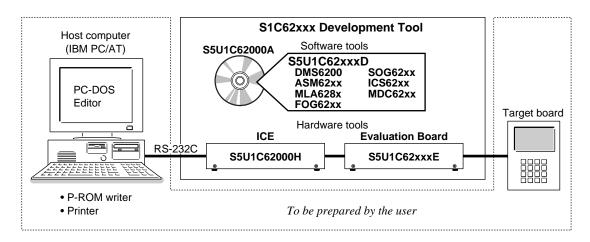
Fig. 2.1 System configuration
